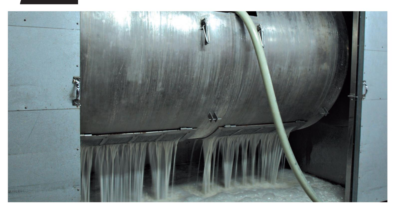
[Washing] The raw ingredient, Indica rice, is thoroughly washed to remove all the bran on its surface, and then soaked in water to absorb sufficient moisture.
