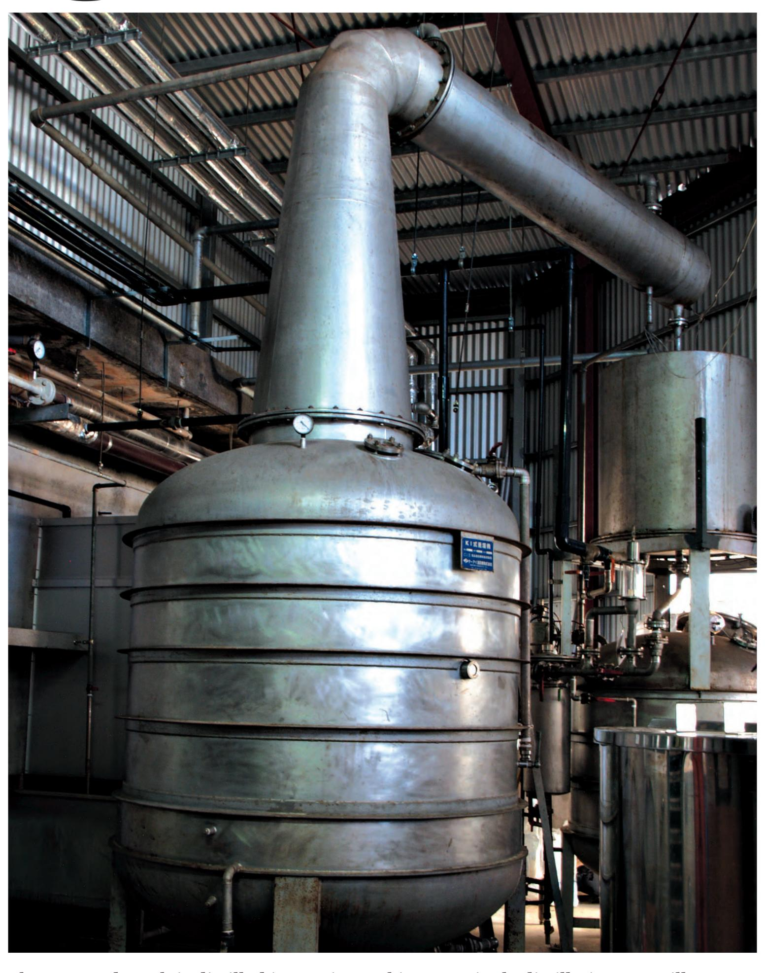
The matured mash is distilled in a unique Okinawan single distillation pot still, to bring out the full richness and aroma of the ingredients.
