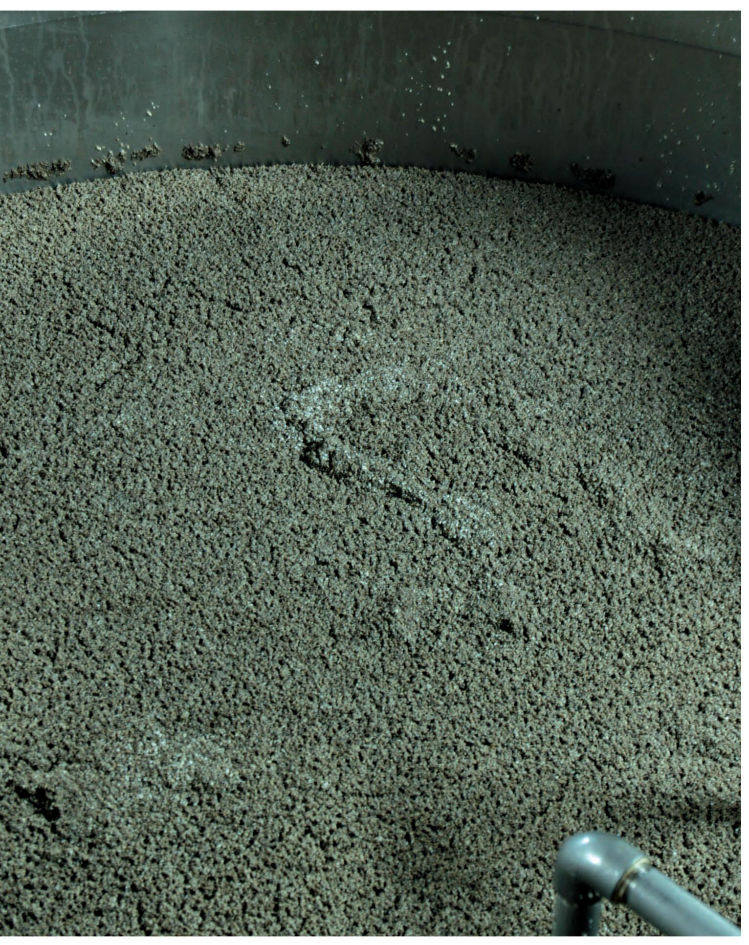
The koji is transferred to the fermentation room and left to mature for one day. Water and yeast are then added to the koji, and fermentation takes place in the mash tank. After about 14 days, the mash ("moromi") reaches an alcohol content of around 18%.
