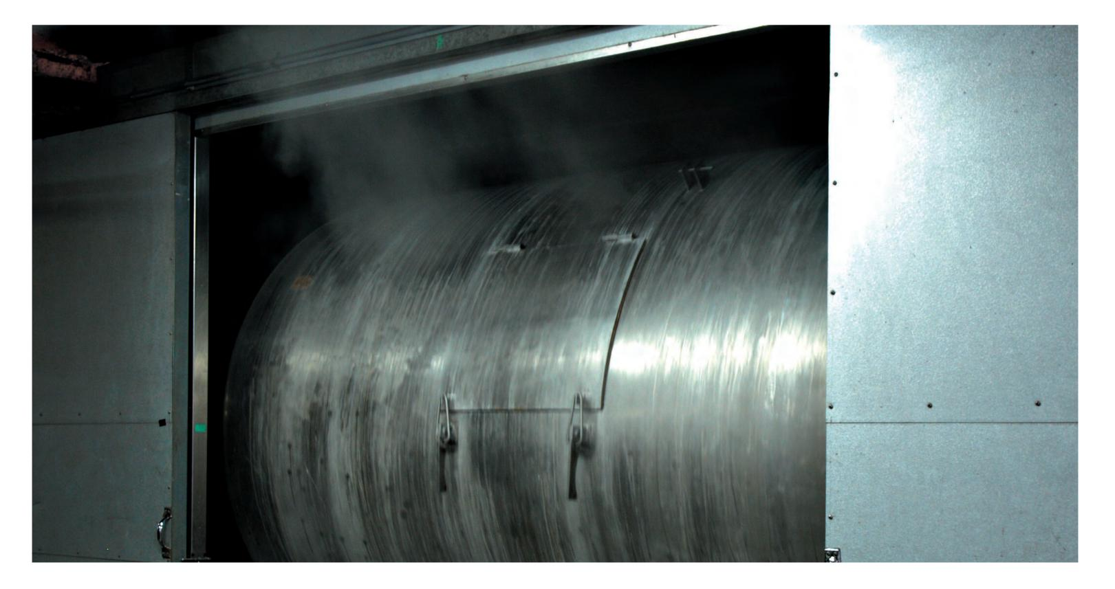
[Steaming] After draining, the rice is steamed in a rotating drum at 120°C for about one hour.
